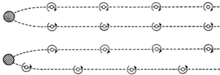
Fig. 32. Double rows of alternating vortices; symmetric (*upper*) and asymmetric (*lower*) arrangements.
