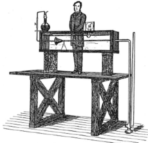
Reynolds' Turbulent flow experimental apparatus
