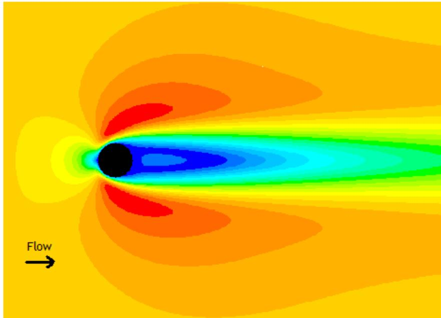
Simulation of Flow over a Cylinder at  $Re = 40$
