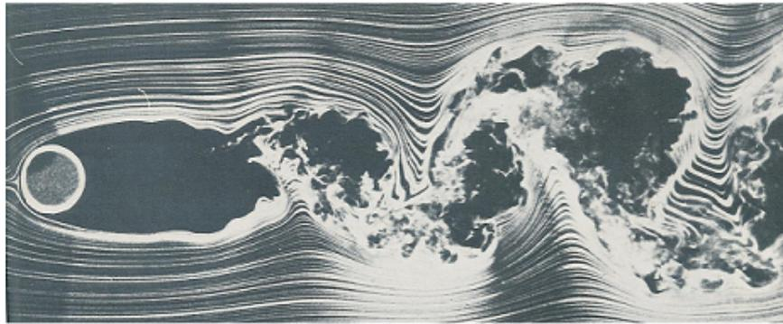
(a) Visualizing turbulent cylinder wake at  $Re = 10000$
