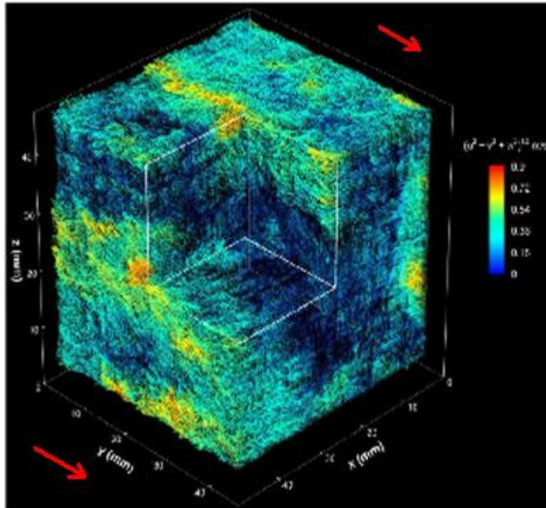
Instantaneous three dimensional velocity distribution of turbulent flow in a square cross-sectioned duct measured using holographic particle image velocimetry (PIV). Color scales indicate velocity magnitude with blue as low and red as high values. Flow is along the arrow marked direction.
