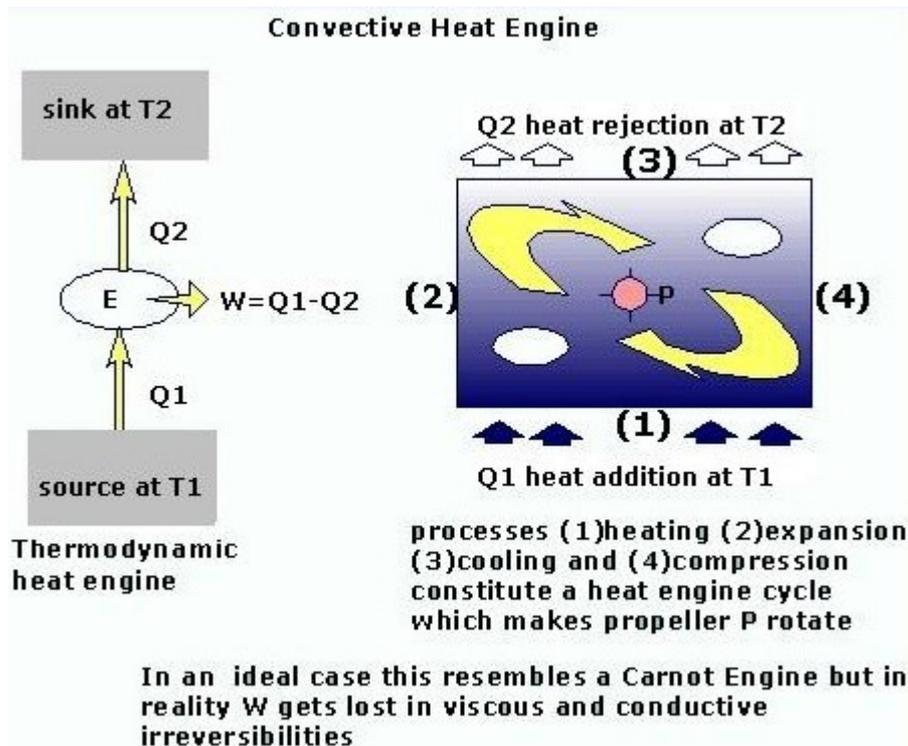
Fig. 1. Convection Carnot Engine Analogue
