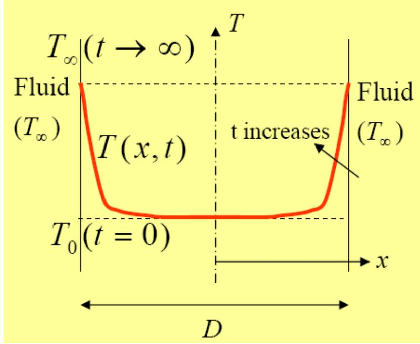
Fig. 1. Schematic of heating a thin plate by hot fluid
