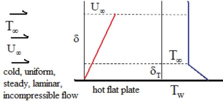
Thin Thermal Boundary Layer Limit ( $Pr \gg 1$ )
