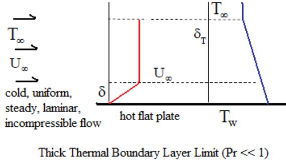
Fig. 1. Schematic for forced convection over flat plate in the thick thermal boundary layer limit
